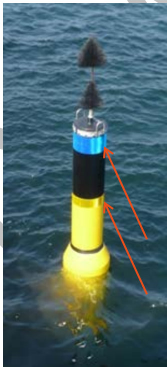
Figure 32 Retroreflective band on a North Cardinal and a West Cardinal buoys (Comprehensive Code)
