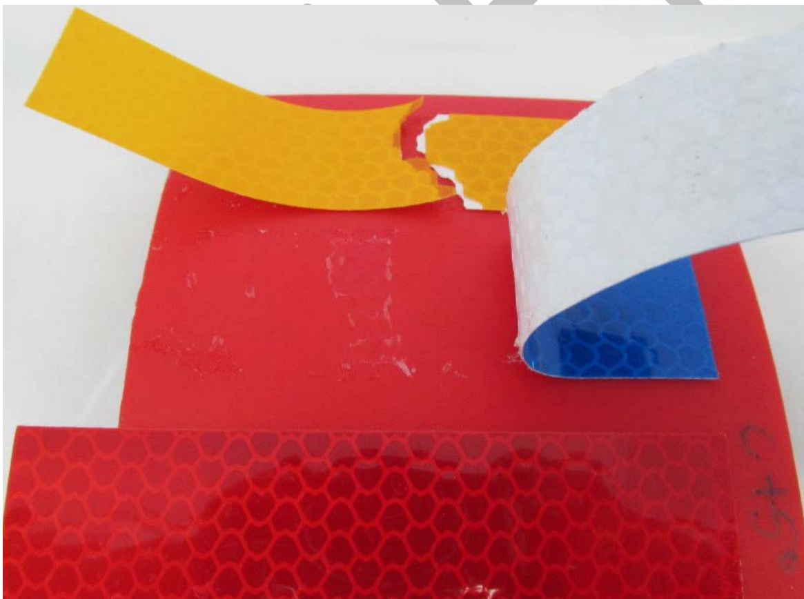
Figure 43 Comparative analysis of adhesiveness of retroreflective sheets applied to plastic buoy material [picture: Solar Simulator Finland Oy]
