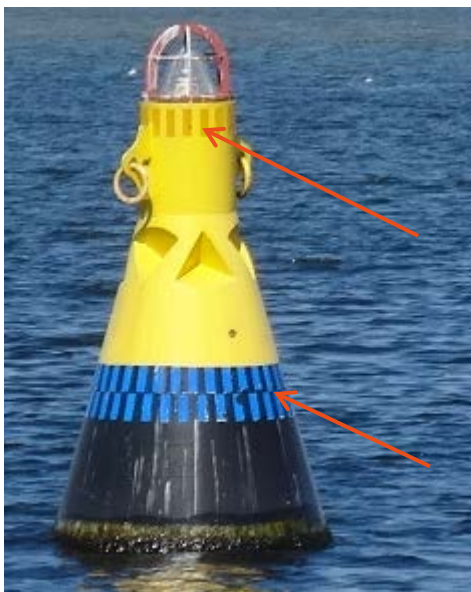
Figure 33 South Cardinal with vertical retroreflective sheets (Comprehensive code)
