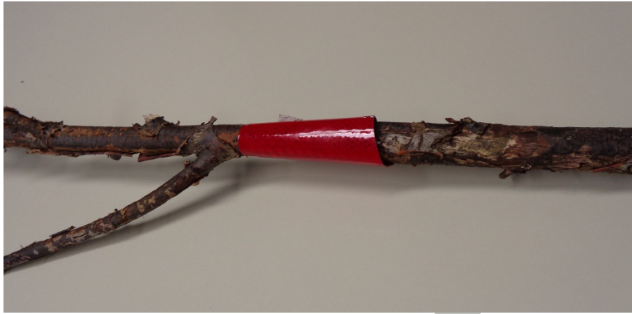
Figure 40 Retroreflective sheet fixed to a withy
