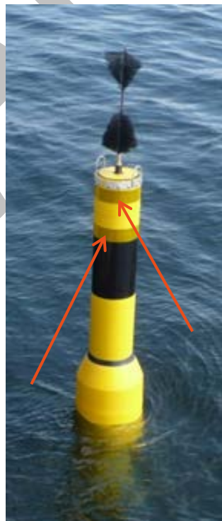
Figure 32 Retroreflective band on a North Cardinal and a West Cardinal buoys (Comprehensive Code)
